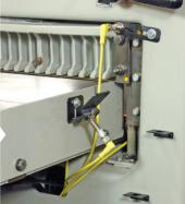
Sensors for clamp, clamp shoe, position and cut if required.
