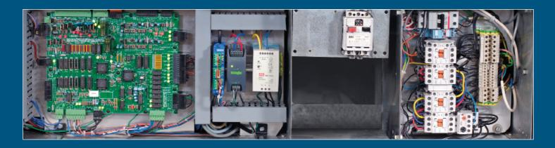
The C&P Microsystems B65 paper cutter control system allows any flywheel cyclical paper cutting machine to be brought to modern standards. The system is a complete clamp/cut control system that can replace an existing control system and is available as an OEM package for new machines. The system does require the installation of a microcut PLUS WS backguage control system for the operator interface.
