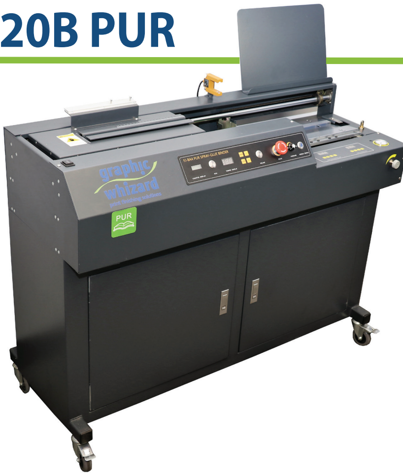
In-line notching, glue application, and nipping station
