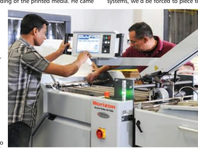
The advanced folder automation and touchscreen control allows ultra-quick set-ups in the Access Direct production facility.
