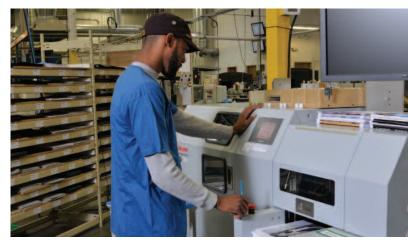
Once the book blocks are created on the Standard Hunkeler line and bound on the Standard Horizon BQ-470 perfect binder, they are loaded into the HT-30 for unattended three-side trimming.
