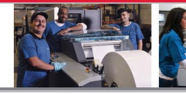
repeatable and more consistent," Mitchell confides. He cites RPI's Standard Horizon AFC-566 Folder with intelligent stacker, in-line with the Hunkeler cutter, as a transformational investment. The folder features a touch-screen control panel, the ability to store up to 200 job settings, and 17 pre-set fold styles. Setups for new jobs can take as few as 14 seconds,
