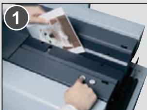
1 Insert the book block and press the start button.
