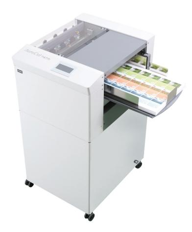
Stable air feed mechanism takes a wide range of paper stocks. Cuts and cross cuts prints in one pass. Elevated feed table separates digital stocks to avoid mis-feedings, damages and roller marks. Density sensor for true double feed detection. 2 single blade margin slitters and 2 double blade gutter slitters are easily adjustable for various stock sizes. InstaSet bar indicates and fixes slitter positions accurately. Intuitive touch screen holds 16 pre-programmed jobs and 40 customized jobs.
