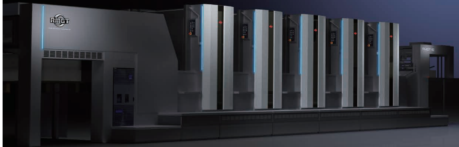
1050ST-5 (1,050 mm Format Straight 5-Color Offset Press)
