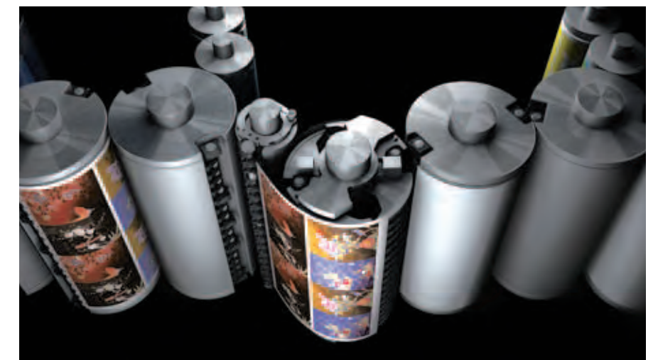
Double/double/single-diameter cylinder perfecting mechanism* * Standard on 8- and 10-color perfectors and optional on 2- to 6-color models
