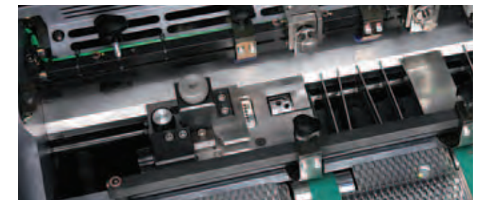
Pneumatic side lay device
