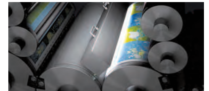
Inter-deck UV curing unit over the impression cylinder
